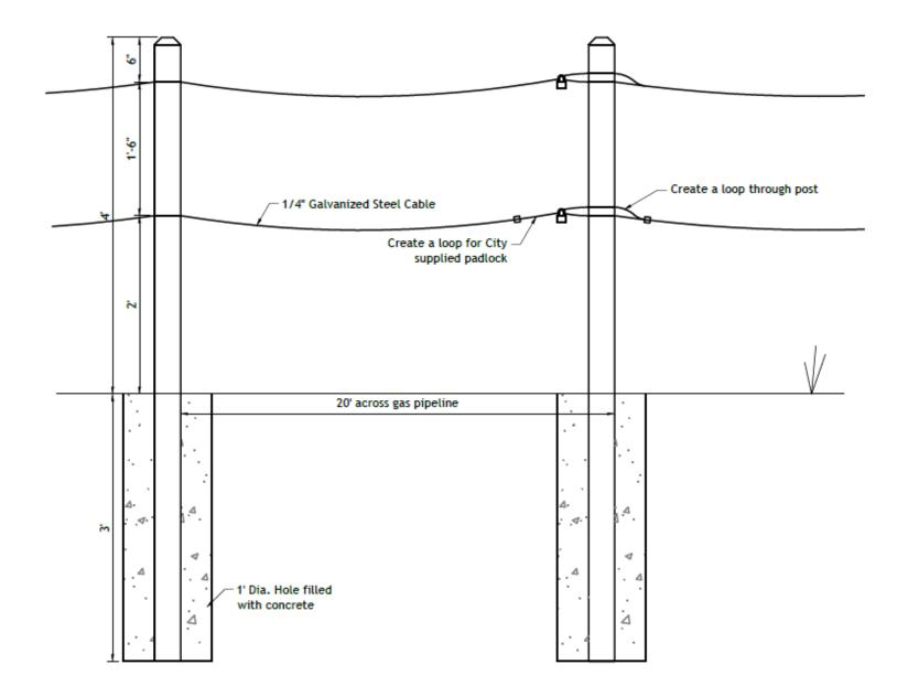
Cable Fence Opening at Pipeline
